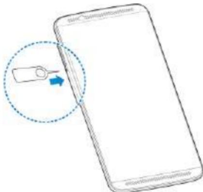
2. Place the nano-SIM/microSDXC card on the tray with the gold-colored contacts facing down. Then carefully slide the tray back into place.
