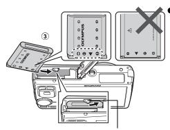
Insert the battery by putting in the ▼ marked side first, with the ⊕ marks toward the end of the camera, the ⊕ marks toward the center of the camera.
