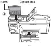
Orient the card, and insert the card straight in. Insert the card until it clicks into place.
