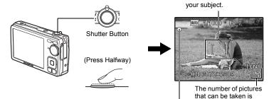
When the focus and exposure are locked, the green lamp lights up, and the shutter speed and aperture value are displayed.
